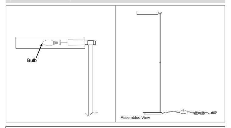
Insert Bulbs (not included) into the socket and rotate it in clockwise to secure. Restore power to the circuit at this time and check for proper lighting operation. Assembly is now complete and the product is ready for use.
