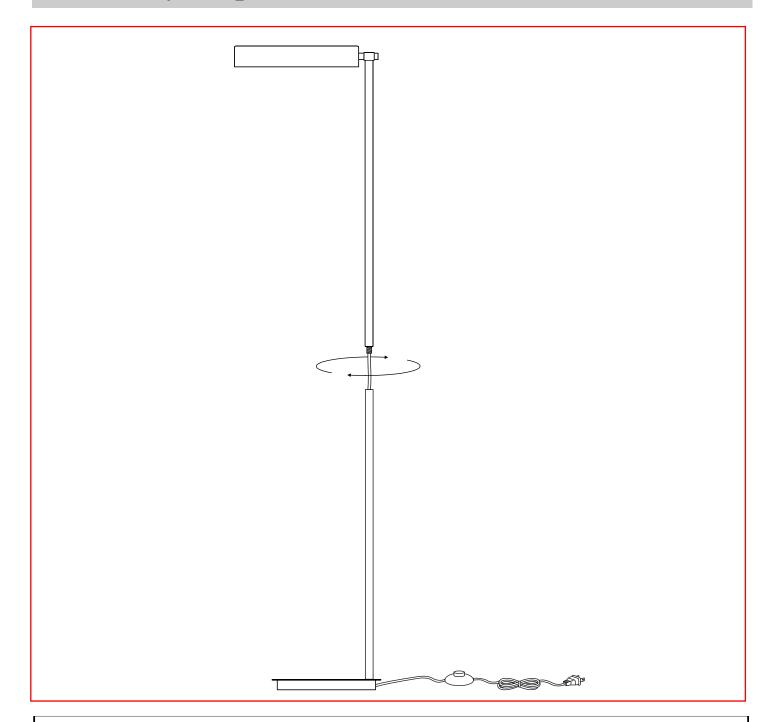
Align stem section on top of each other and rotate upper section clockwise to secure.
